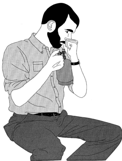
Figure 2. After a normal exhalation (eliminating the dead-space portion of a breath), the subject places the end of the Teflon ® collection tube of the SBC in his mouth and opens the canister valve to fill the volume with 1 litre of the lungs' expiratory reserve. Because the canister is initially evacuated ( < 50 \mu\text{mHg} ), the sample is collected until it comes to atmospheric pressure.
